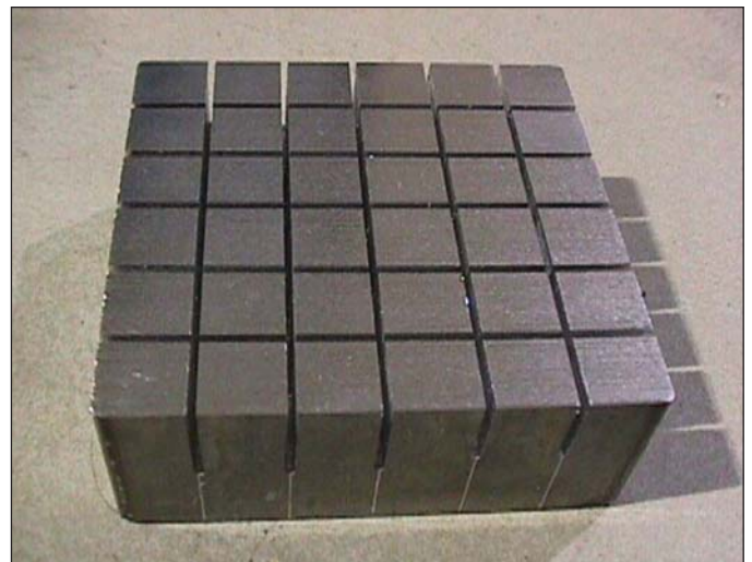
Fig. 2. The effect of microstresses is minimized by utilizing 36 d_0 samples in which macrostresses are relaxed by the cross-cutting technique shown.
