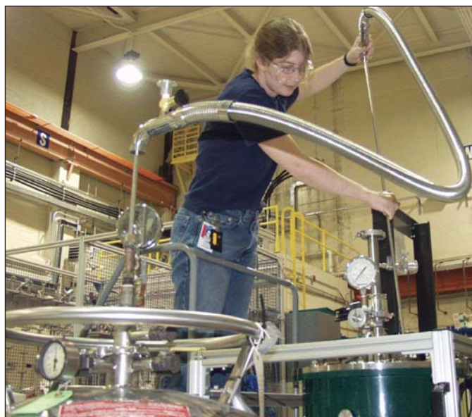
Fig. 4. Rachel Anderman (NCNR) fills the new 9T horizontal field superconducting magnet with helium.
