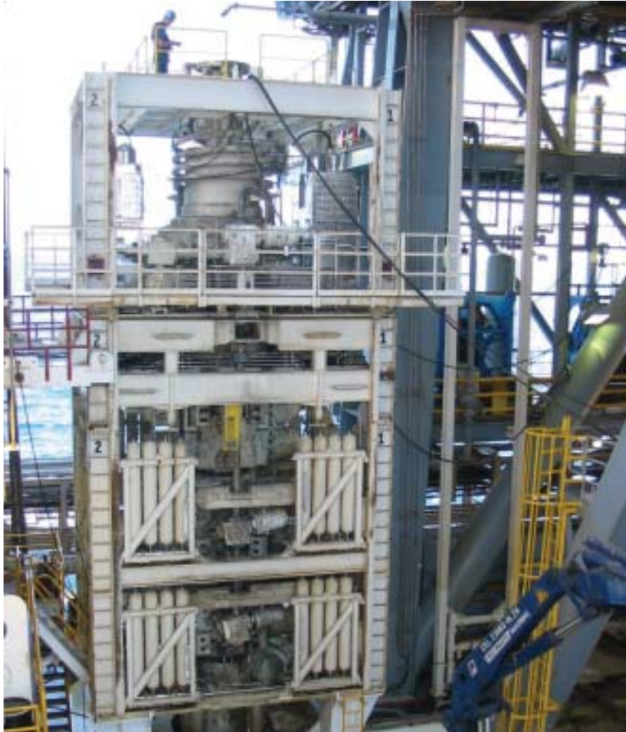
Above: A blowout preventer (BOP) used for deepwater drilling projects. Note the man standing on the top.
