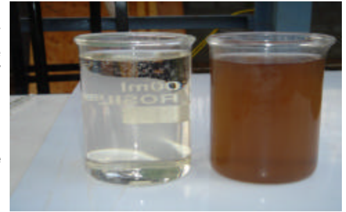
Outlet and Inlet to the VSEP Plant
