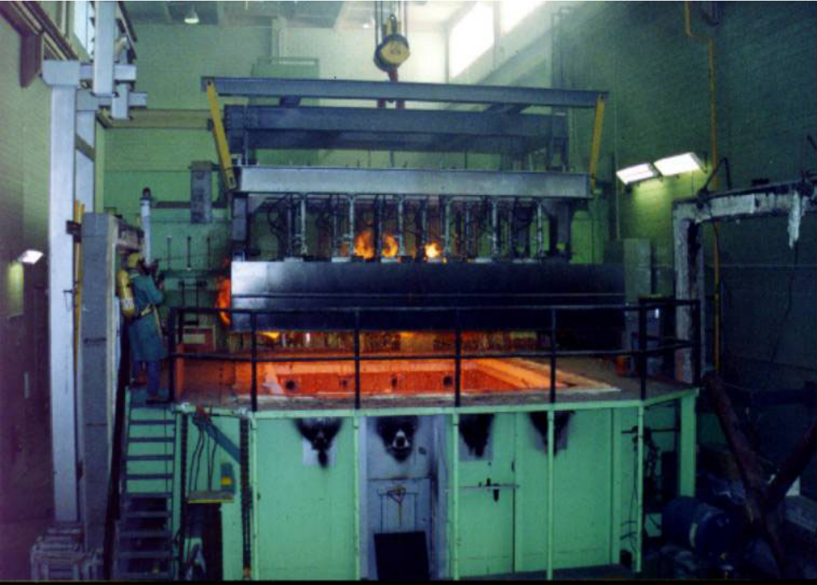
Figure 6. Photograph of modern floor testing furnace (Kodur)
