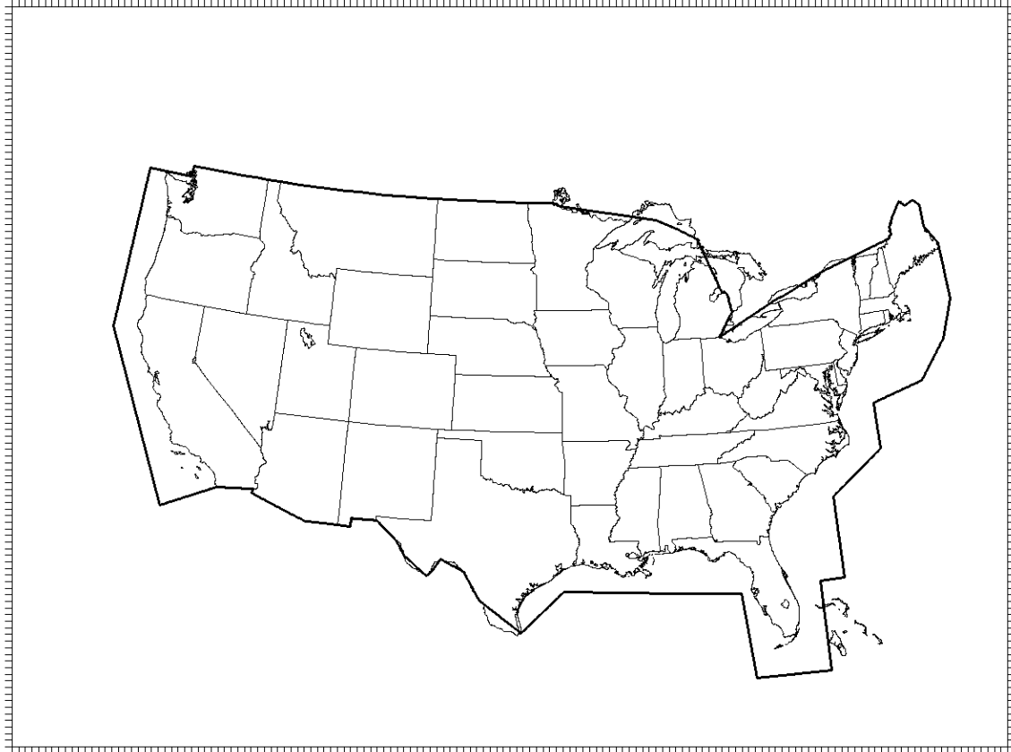
Figure 1. RUC-2 domain. Tics on the edges of the frame identify the model grid lines; dark outline around continental U.S. denotes the total domain of the AIRMETS.
