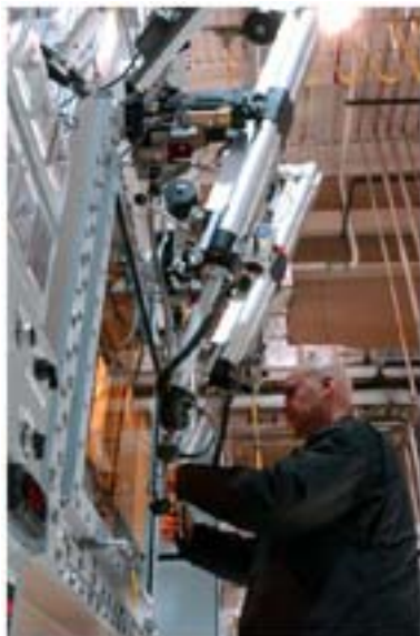
Chemistry division employee Louie Salazar operates the hot cell manipulators in the new Isotope Production Facility at the Los Alamos Neutron Science Center.
