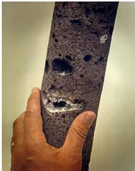
This basalt core sample from between 200 and 400 feet below the surface contains air pockets in which calcite material crystals grew.
