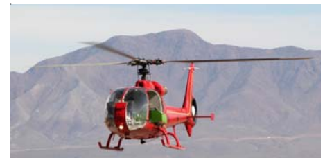
The green box on the right of the helicopter contains a laser-based hydrocarbon detection unit to be field tested at DOE's Oilfield Testing Center.
