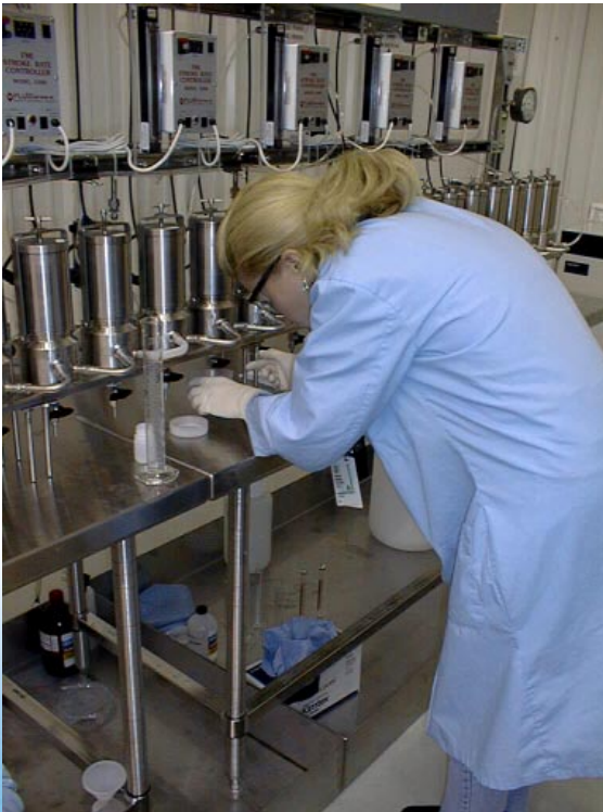
These three photos show scientists researching various types of centrifugal contactors, a central component of the aqueous method of nuclear fuel processing.
