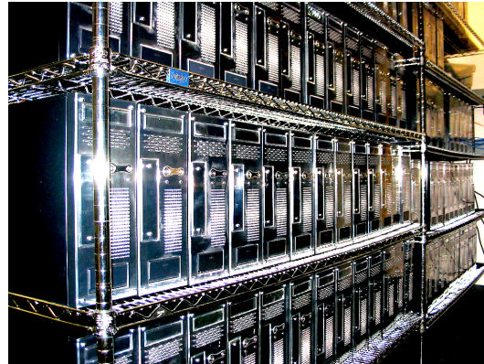
A 200-processor Beowulf cluster enables the Land Information System (LIS) to model the globe at the same resolution as NASA satellite observations (Photo credit: Yudong Tian, GSFC).
