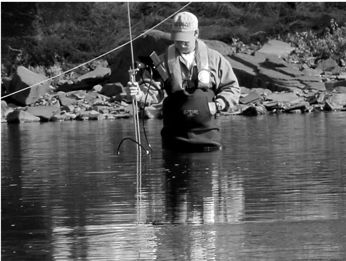
USGS hydrographer making a wading discharge measurement at Pee Dee River below Lake Tillery, North Carolina.
