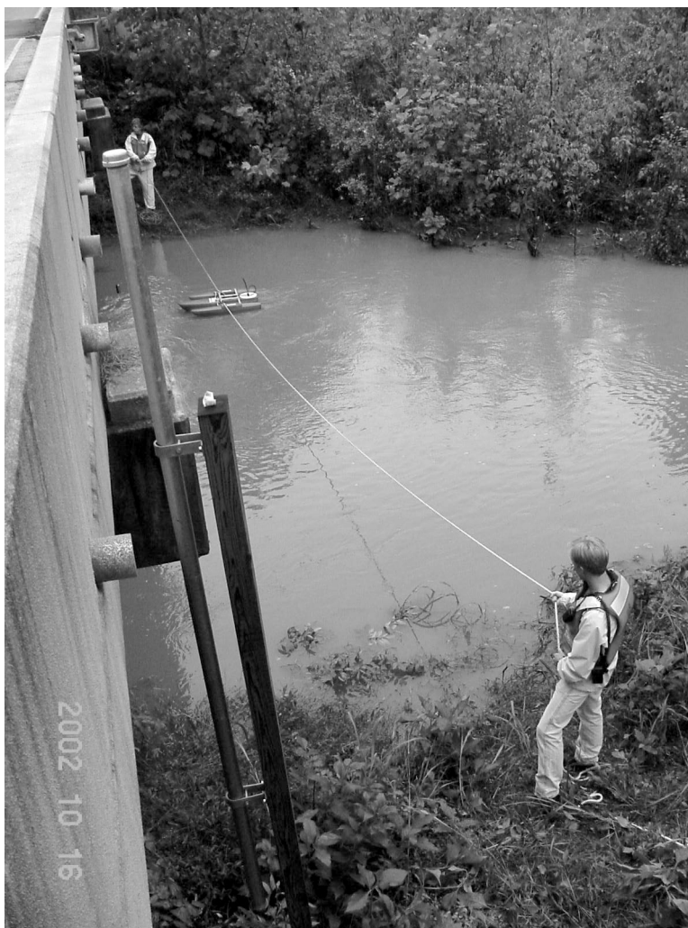
Streamflow measurement using Acoustic Doppler Current Profiler at Four Mile Creek, North Carolina.
