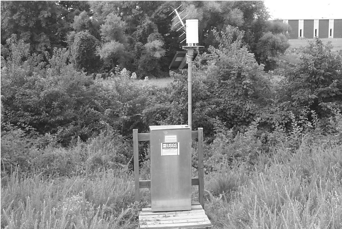
Gaging station and raingage at Ryan Creek below US 220 at Greensboro, North Carolina.
