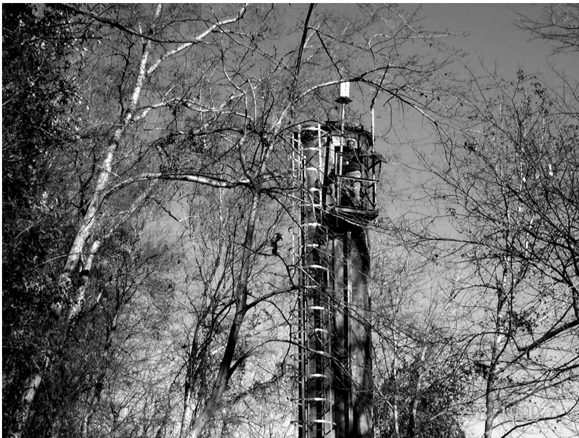
Gaging station at Cape Fear River at William O. Huske Lock near Tarheel, North Carolina.
