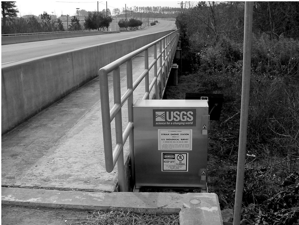
Gaging station at Mallard Creek below Stony Creek near Harrisburg, North Carolina.
