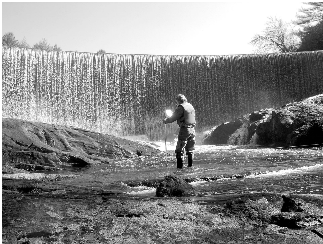
USGS hydrographer making a wading discharge measurement below dam at Cullasaja River near Highlands, North Carolina.
