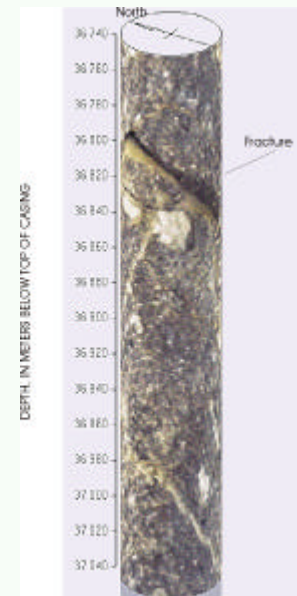
Figure 2. The two dimensional image can be rolled into a "virtual core," and the core can be rotated using post-processing software.
