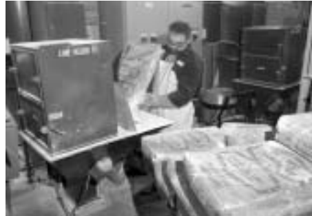
4. LIME is added after aeration (no. 3) and before retention (no. 6) to raise the pH and soften the water. Feeding lime into the hopper is Steve Barcelo.
