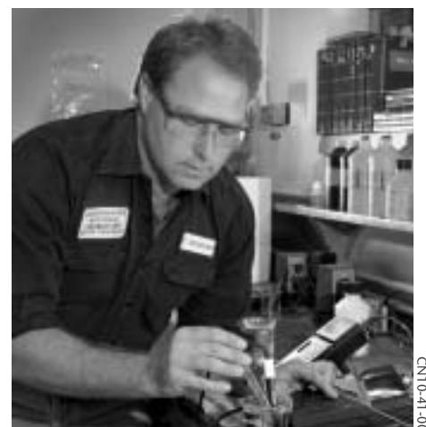
13. TESTING THE QUALITY OF BNL'S DRINKING WATER at the WTF is Tom Boucher. The Lab's drinking water is tested in various locations weekly, monthly, quarterly, semi-annually, and annually, depending upon the test. Test samples are analyzed by certified laboratories, and results are reported to the Suffolk County Department of Health Services, which conducts its own annual tests of public water systems in the county. BNL results are also delivered to BNL's Environmental & Waste Management Services Division, which ensures that the Lab's water is in compliance with all applicable regulations. The results are summarized in this publication, the Lab's annual Water Quality Consumer Confidence Report.
