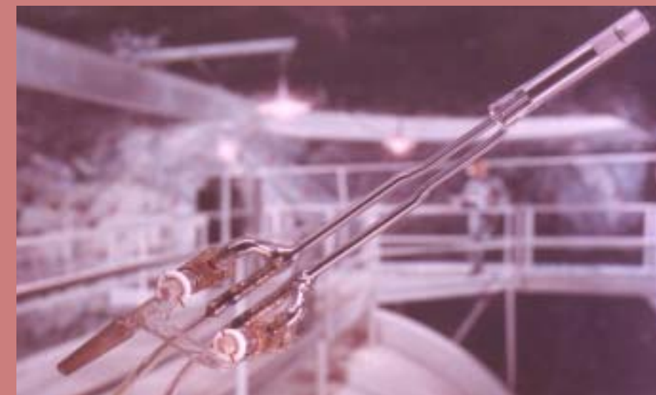
The very small number of argon-37 atoms created by solar neutrino capture are first extracted from the large tank (background) containing about 10^{31} chlorine-37 atoms and then transferred into a proportional counter (foreground) with an active volume of approximately 0.5 cubic centimeters.
