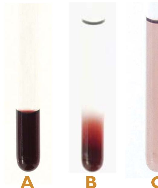
Soluble in a reagent (A), the new catalyst remains soluble when another reagent is added (B). As the reaction goes on and the product builds up (C), the catalyst precipitates from the mixture as an oil (D), which
