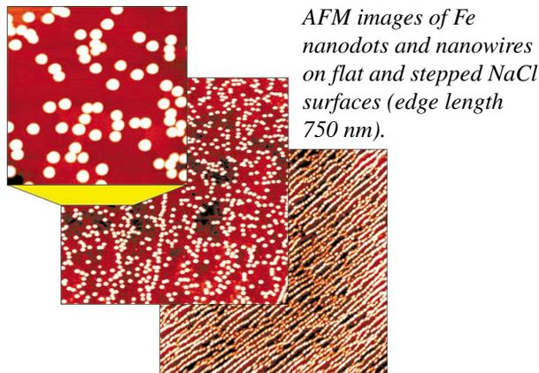
*AFM images of Fe nanodots and nanowires on flat and stepped NaCl surfaces (edge length 750 nm).*
