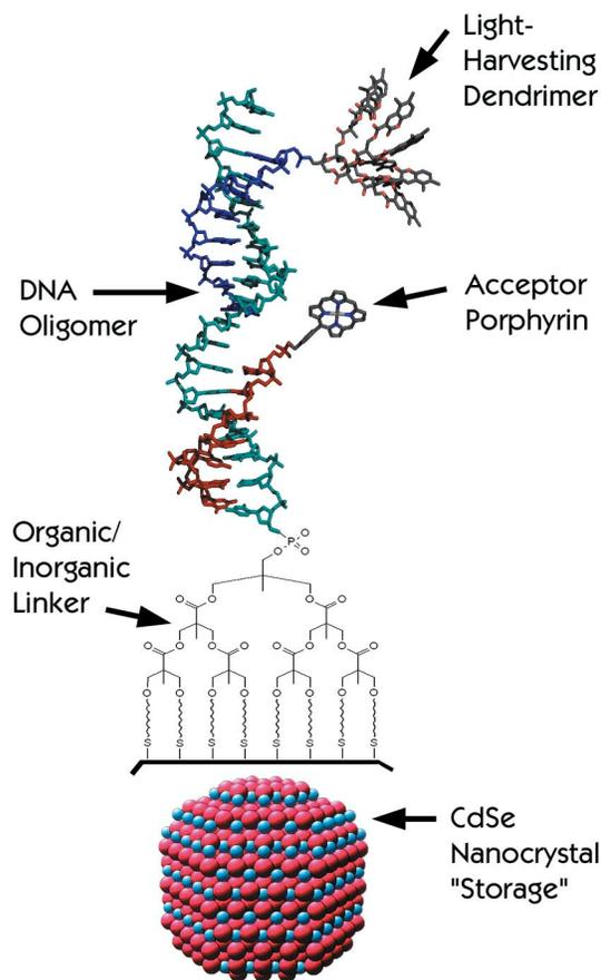
*Nanoscale building blocks can be combined to make novel functional devices, such as this design for a photosynthetic reaction center with integral semiconductor storage.*
