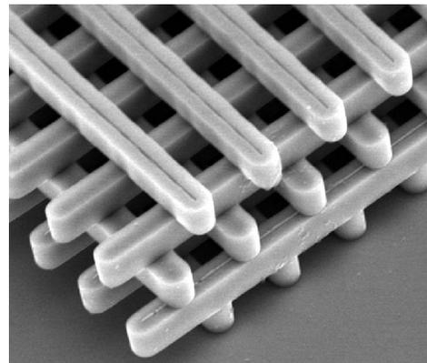
*Photonic lattice constructed of 1.2- $\mu\text{m}$ -wide silicon "logs."*
