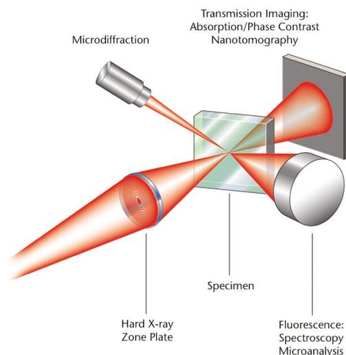
*The CNM’s nanoprobe beamline at the Advanced Photon Source will focus hard X rays down to a spot size of 30 nm or smaller.*
