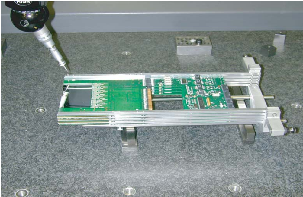
Figure 2.4: Assembled detector package on survey bench without trigger scintillator.
