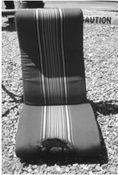
(b) Seat - 25 kW sand burner
