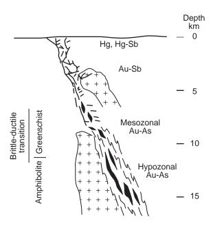
**Figure 1.** Schematic representation of shear-zone setting of low-sulfide gold-quartz veins and related deposits. Mod-ified from Groves and others (1998), and McCuiag and Kerrich (1998).
