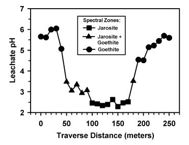
**Figure 3.** Surficial mine-waste leachate pH versus distance along a mine-waste pile traverse. Each spectral mineral zone is denoted by a different symbol. Note that the pH is lowest in the jarosite spectral zone. After Swayze and others (2000b).
