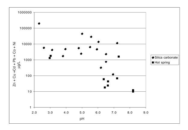
**Figure 3.** The sum of the base metals Zn, Cu, Cd, Pb, Co, and Ni versus pH (Ficklin plot) for mercury mine drainage from silica-carbonate and hot-spring type mercury deposits.
