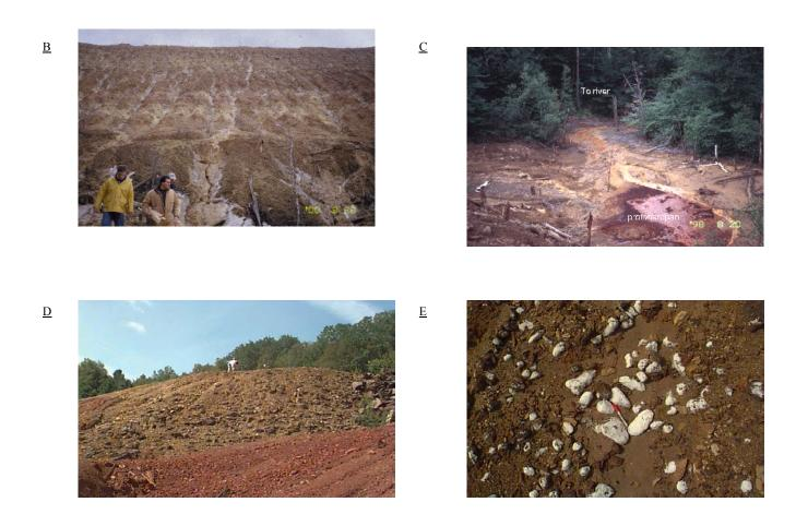
**Figure 3.** <u>B</u>, Deeply eroded, bare north slope of TP1 above seeps. <u>C</u>, Ochres precipitating at seeps at base of TP1. <u>D</u>, TP3-D (yellow-brown pile in center of photo) and TP3-E (red pile in foreground). <u>E</u>, Close-up of melanterite-rozenite "snowballs" on weathered ore that litters TP3-F. Salts are observed on hot, dry days; they disappear when it rains.
