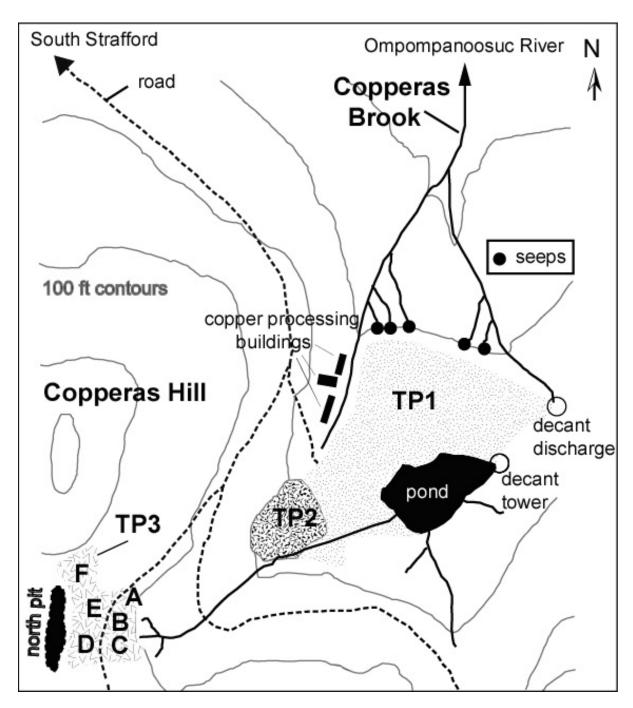
Figure 3. Mine waste and flotation tailings at the abandoned Elizabeth copper mine, VT. A, Site map showing the relative size and distribution of solid materials that impact Copperas Brook. TP1 and TP2 represent flotation tailings from 20<sup>th</sup> century mining. TP3 consists of heterogeneous piles of mine waste from 19<sup>th</sup> century mining and copperas processing. See table 8a for descriptions of individual piles.
