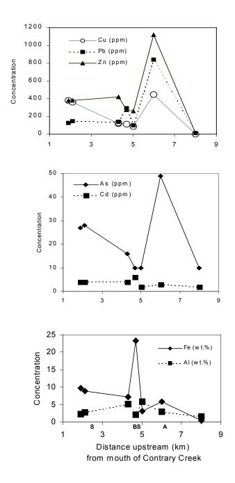
Figure 6. <u>B</u>, Metal concentrations in <80 mesh stream sediments along Contrary Creek as it flow past abandoned mines. See localities 1-8 on fig. 6A for sample locations. S, Sulfur mine; BS, Boyd Smith mine, A, Arminius mine. The Arminius mine near the headwaters of the creek (at 6 km) inputs significant amounts of base metals and arsenic; the Boyd Smith mine area contributes the most iron. Relative to the headwaters area above the mines, all metals increase downstream.
