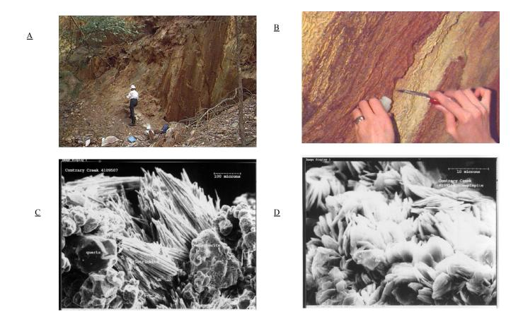
Figure 4. Efflorescent salt minerals along a pit wall.  $\underline{A}$ , Salts form colored vertical bands on outcrops under a protected overhang.  $\underline{B}$ , Sampling techniques.  $\underline{C}$ , Secondary-electron SEM image showing needles of halotrichite intergrown with melanterite and quartz.  $\underline{D}$ , Secondary-electron SEM image of copiapite crystals (yellow mineral shown in  $\underline{B}$ ).
