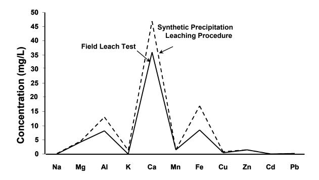
**Figure 1.** Comparison of leaching results of a < 2 mm fraction mine-dump composite from the Yukon mine near Silverton, Colorado. The dashed line represents results from the Synthetic Precipitation Leaching Procedure and the solid line represents results from the Field Leach Test. Modified from Hageman and Briggs (2000).
