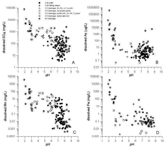
Figure 4. Dissolved concentrations of A) sulfate (SO<sub>4</sub>), B) arsenic (As), C) manganese (Mn), and D) iron (Fe) versus pH in drainage from polymetallic vein deposits in the Coeur d'Alene mining district, in the Colorado Mineral Belt, and in the Humboldt Basin in northern Nevada.
