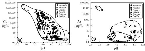
**Figure 4.** Comparison of filtered mine drainage waters with natural background waters. Data outlined by solid lines are mine drainage; data outlined by dashed lines are natural backgrounds. a Cu vs. pH. The general negative slope of the data is typical of most divalent metals. b. As vs. pH. Note that many of the natural background samples have higher As concentrations than the mine drainage samples.
