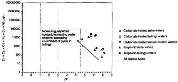
**Figure 3.** Ficklin plot showing some compositions of mine waters, tailing waters, and a natural water draining carbonate-hosted and jasperoid-rich MVT deposits. The plot is used to compare the sum of dissolved base metals (Zn, Cu, Cd, Pb, Co, and Ni) to pH and illustrate how mine drainage chemistry can vary as a function of the mineral deposit type. Figure is from Plumlee and others (1999).
