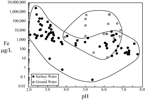
**Figure 2.** Fe versus pH for filtered mine drainage samples from Besshi-type deposits. Note that ground waters (seeps) from this deposit type have elevated Fe concentrations at comparable pH values relative to surface waters because of the higher solubility of ferrous iron found in ground waters.
