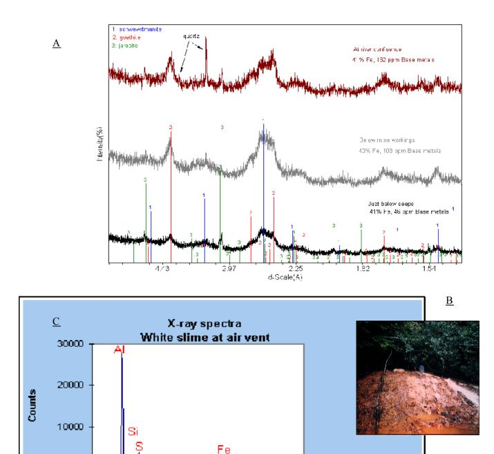
Figure 5. Ochre minerals. A, XRD patterns of iron-rich precipitates in Copperas Brook below the Elizabeth mine (fig. 3). Note that base metals incorporated in these ochres increase downstream from the mine workings. B, White slime at air vent, with a mount of white and red-orange precipitates that engulf leaf litter. C, Energy-dispersive spectrum of white slime analyzed by SEM shows that it is aluminum-rich, with minor silicon, iron, and sulfur.
