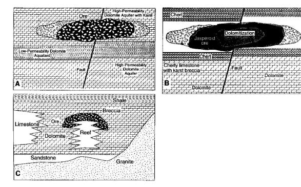
**Figure 2.** Schematic cross-sections showing geologic features of various platform carbonate deposits, from Plumlee and others (1999). The cross sections reflect concepts presented by Leach and Sangster (1983) and references therein: A. Central Missouri district, B. Tri-State district, and C. Viburnum Trend.
