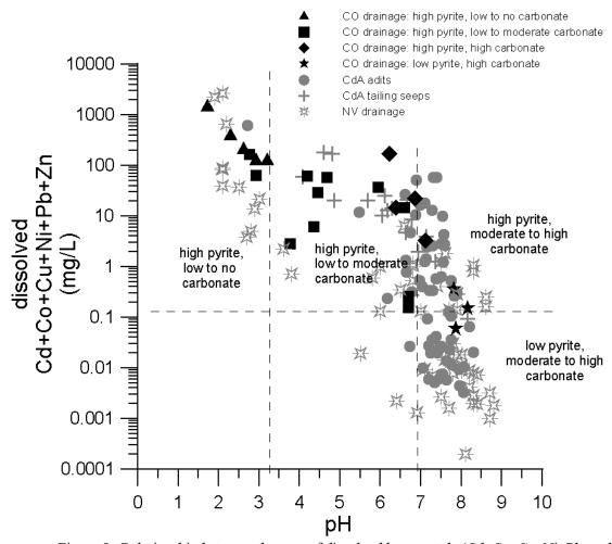
Figure 5. Relationship between the sum of dissolved base metals (Cd, Co, Cu, Ni, Pb, and Zn) and pH in mine drainage from diverse deposit types in the Colorado Mineral Belt and from polymetallic vein deposits in the Coeur d'Alene mining district and in the Humboldt Basin in northern Nevada.
