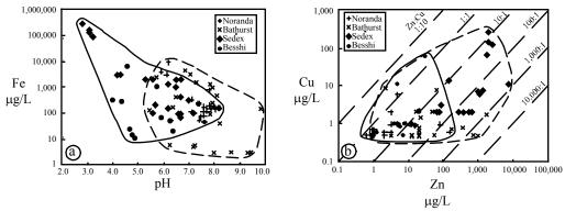
**Figure 3.** Natural background geochemical data for filtered ground and surface waters around massive sulfide deposits. a. Fe vs. pH. Data outlined by solid line are from deposits exposed at the surface; data outlined by dashed line are from buried deposits. b. Cu vs. Zn. Dashed lines represent Zn:Cu ratios (mass basis). Note that waters from Zn-rich deposits (Sedimentary-exhalative and Bathurst) range to higher Zn:Cu ratios than Cu-rich deposits (Noranda and Besshi).
