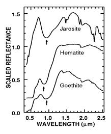
**Figure 2.** Spectra of some iron-bearing secondary minerals. Note the different shapes of the spectra, which are diagnostic for mineral identification. After Dalton and others (2000).
