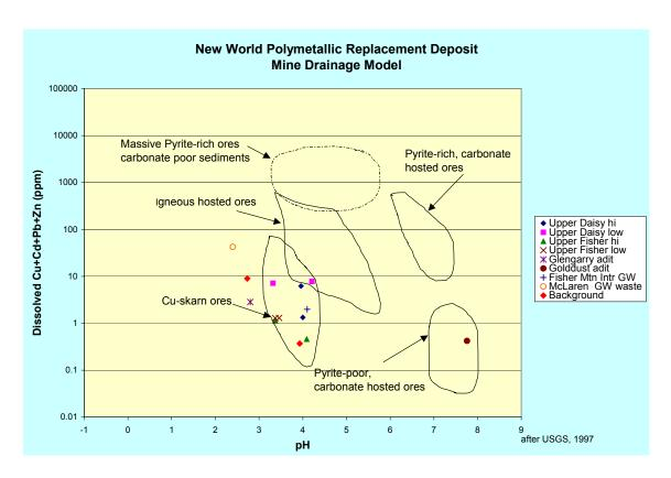
**Figure 4.** New World Polymetallic Replacement/Skarn deposit mine drainage model, based on USGS geoenvironmental model approach.
