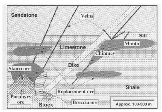
**Figure 1.** Generalized conceptual model for the geologic setting of high-temperature, carbonate-hosted and related deposits associated with igneous intrusions. (From Plumlee and others, 1999, figure 19.18)
