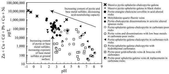
**Figure 1.** Ficklin plot of the sum of the base metals Cd, Co, Cu, Ni, Pb, and Zn versus pH illustrating the variation of mine drainage chemistry as a function of the geologic characteristics (type) of specific mineral deposits. Modified from Plumlee and Nash (1995), and Plumlee (1999).
