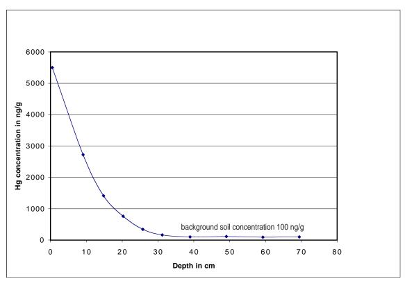
**Figure 2.** Profile of mercury concentration in soil impacted by release of particulate mercury and vapor from mercury mines in the New Idria mercury district, California.
