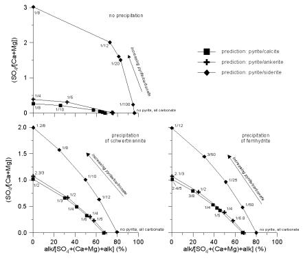
Figure 6. Predicted relationships between the ratio of sulfate (SO<sub>4</sub>) to the sum of dissolved calcium (Ca) and magnesium (Mg) and normalized alkalinity (alk) for various ratios of reacting pyrite to carbonate (i.e., calcite, ankerite, or siderite) considering no precipitation of Fe or precipitation of schwertmannite or ferrihydrite.
