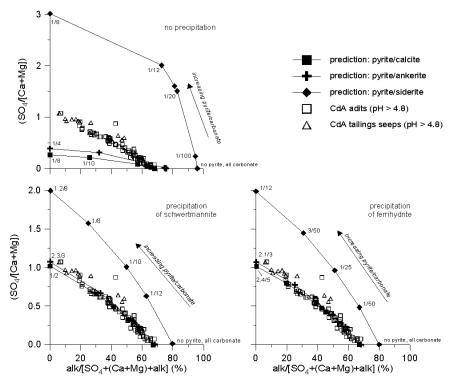
Figure 8. Comparisons between the predictions presented in Figure 6 and the composition of drainage from adits and tailings piles in the Coeur d'Alene (CdA) mining district.
