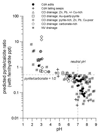
Figure 10. Comparisons between the predicted ratios of reacting pyrite to calcite, considering precipitation of ferrihydrite and calculated as pyritic  $SO_4/(Ca + Mg)$  in drainage, versus the pH of drainage from polymetallic vein deposits in the Coeur d'Alene mining district, in the Colorado Mineral Belt, and in the Humboldt Basin in northern Nevada.
