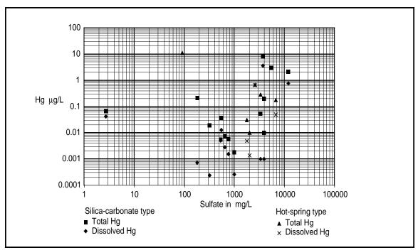
**Figure 5.** Mercury concentration in mercury mine drainage from silica-carbonate type and hot-spring type mercury deposits.
