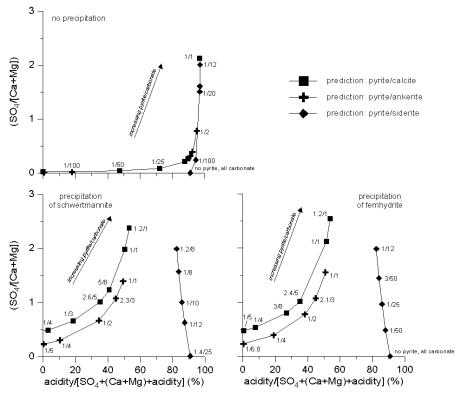
Figure 7. Predicted relationships between the ratio of sulfate (SO<sub>4</sub>) to the sum of dissolved calcium (Ca) and magnesium (Mg) and normalized acidity for various ratios of reacting pyrite to carbonate (i.e., calcite, ankerite, or siderite) considering no precipitation of Fe or precipitation of schwertmannite or ferrihydrite.
