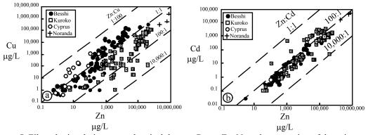
**Figure 5.** Filtered mine drainage geochemical data. a. Cu vs. Zn. Note the separation of deposit types by Zn:Cu ratio (mass basis), which reflects primary differences in deposit types. b. Cd vs. Zn. Note the overlap among deposit types in terms of Zn:Cd ratios (mass basis), which reflects the common source control of Cd as a trace element in sphalerite.
