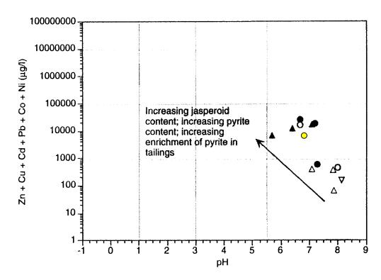
**Figure 5.** Ficklin plot for platform carbonate deposits showing data for Austinville, compared to data for other platform carbonate deposits.
