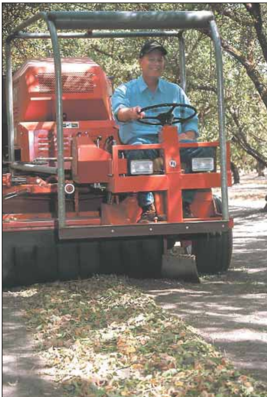
Allen F. Johnson sweeps almonds into windrows, to be collected by a harvester.
