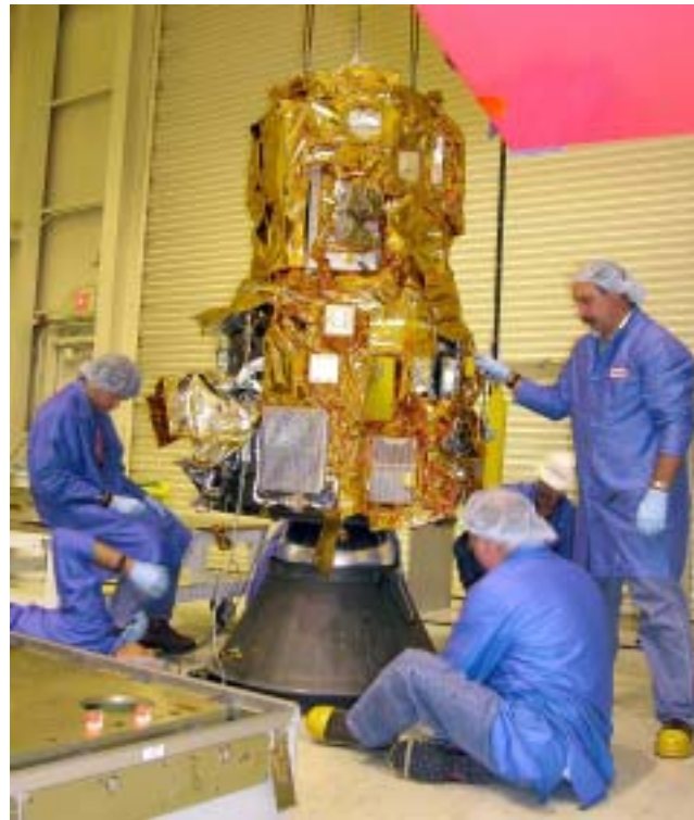
AT VANDENBERG AIR FORCE BASE in California, Orbital Sciences technicians observe closely the movement of the DART (Demonstration for Autonomous Rendezvous Technology) flight demonstrator as it is lowered onto a stand. The spacecraft was developed to prove technologies for locating and maneuvering near an orbiting satellite.
