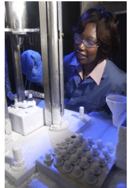
Marceia Clark-Ingram, a Marshall materials engineer, loads a sample into the Ambient Impact tester at the Materials Combustion Research Facility.
