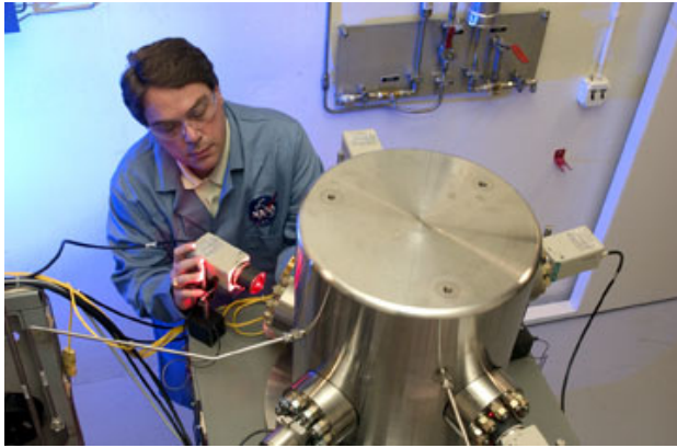
Steve Herald, lead engineer, adjusts a camera that collects data from the Marshall Center's new Heated Promoted Combustion tester.
