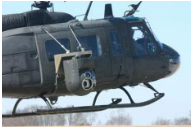
A U.S. Army Huey helicopter, left photo, uses a gimbal-mounted imaging system to target a NASA T-38 aircraft, right photo, during engineering and feasibility tests for tracking a Space Shuttle ascent.
