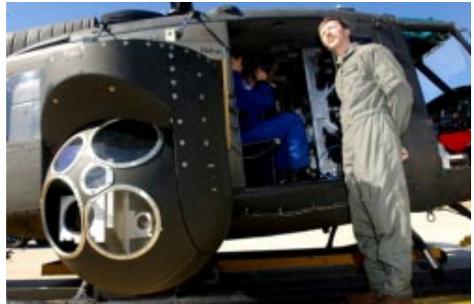
Tim Ricks, senior project engineer for captive flight tests, stands near “Fat Boy,” the gimbal system that holds an array of photographic equipment used in recent imaging tests at the Marshall Center.
