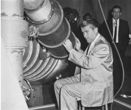
Wernher von Braun tries out a "floating platform" in 1961, at the Marshall Manufacturing Engineering Lab in a test to help determine how future astronauts will perform maintenance tasks in space.
