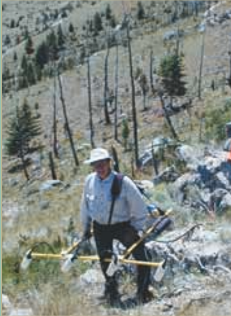
Dr. Roman Pasteka searches for unexploded ordnance on the ridge of Limestone Hills Training Range, Montana, aided by a “quad-sensor, optically pumped cesium vapor magnetometer.”
