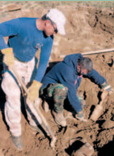
Jerry Krieger and Jeffrey Kennedy (right) conduct magnetometry surveys at a former Camp Edwards, Massachusetts, training range to locate sub-surface munitions.
