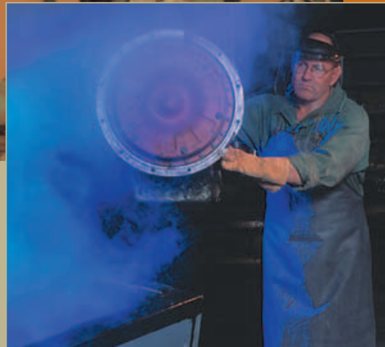
Sergeant 1st Class James Dulin removes a track vehicle transmission from the aqueous parts washer at the National Guard’s maintenance facility on North Ft. Hood, Texas. Hot water replaces solvents to clean parts and reduce waste.
