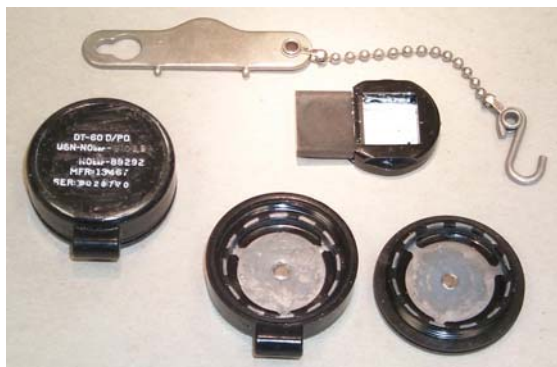
Figure 8. DT-60 battlefield dosimeter. (Top: Opener, Left: Unopened, Right: Disassembled).
