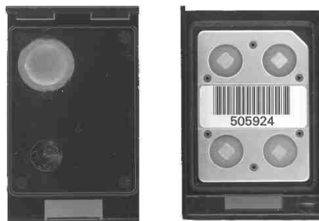
Figure 1: DT-648 Open holder with TLD card inside
