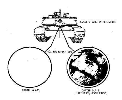
Figure 1. Crazing Effect Of Laser Radiation In Glass
