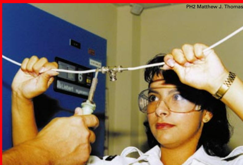
YNSR Mary McLoyd of the Naval Safety Center illustrates a technique that will launch molten solder in your face.
