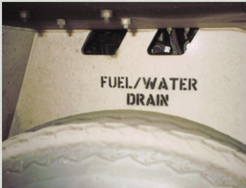
Even though location of the fuel-water separator is painted on the tractor and identified on the pre-op card, most operators don't know where the item is. (It's located on the engine side of the right-front wheelwell.)
