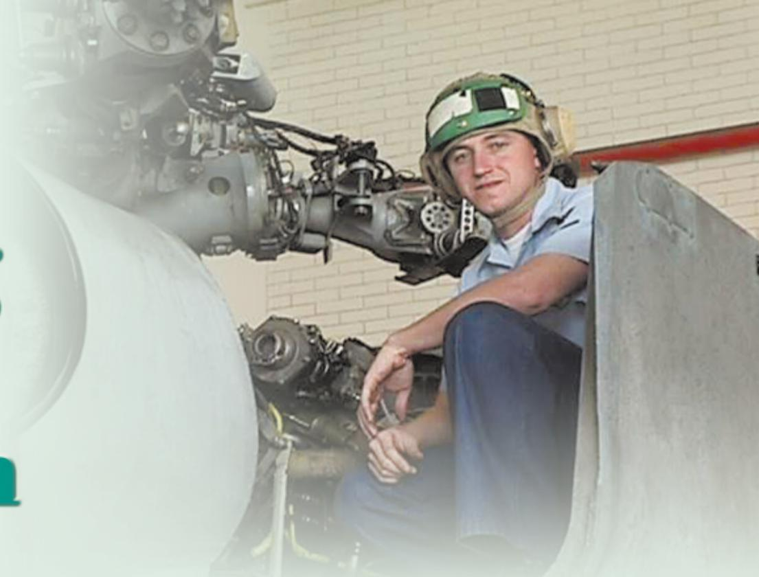
**T**he engine cowling on an SH-60B, like those of most helicopters, is also a platform when it is open. Maintainers and pilots stand on it to do maintenance, preflight and other inspections. Engineered to hold two persons with a combined weight of 400 pounds, this platform should have accommodated my 150 pounds without a problem, but it let me down—a long way down.
