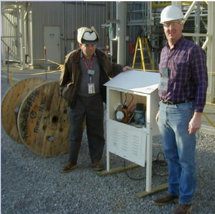
A particle size analyzer deployed at Fernald which is currently used to supplies airborne particulate concentration and size data at the waste pits, the soil dryer and at buildings being removed. [see Project #74050, renewal of #59882]
