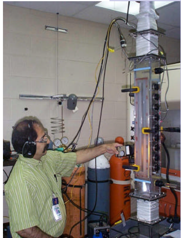
Experimental apparatus allows testing of the effect of electric and acoustic fields on flowing aerosols in 10-cm (4-inch) square duct. Size distribution and concentration of aerosol are measured to determine effectiveness of agglomeration. [see Project #65328]
