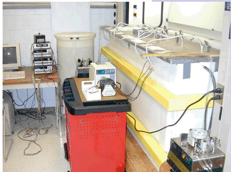
Photographs of 3-D large tank experiment. The experiment was designed to simulate the in-situ remediation of TCE residually saturated in sand aquifer. Reaction occurring in the sand aquifer is subject to monitoring for concentration of TCE, permanganate and chloride as a reaction product. [see Project #73745, renewal of #54585]
