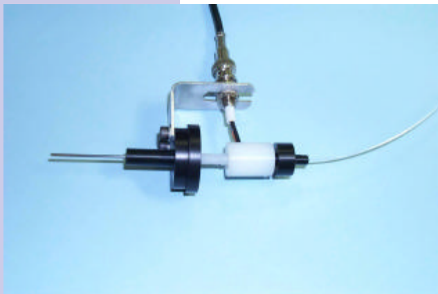
Prototype coaxial fiber/electrode REMPI probe. [see Project #70050]
