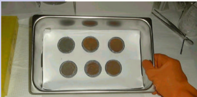
Preparation of Contaminated Steel Coupons. [see Project #64907]
