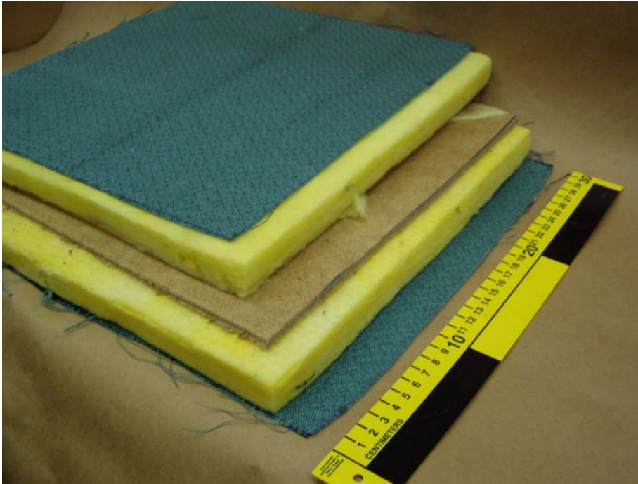
Figure 44. Combustible workstation side panel components
