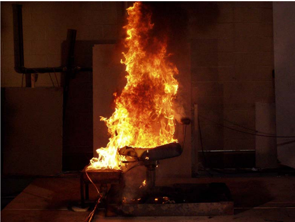
Figure 55. Office chair, approximately 150 s after ignition
