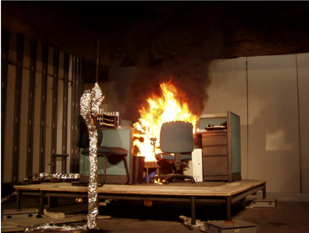
Figure 68. Single workstation, 150 s after ignition
