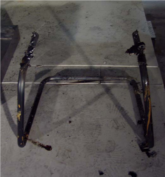
Figure 50. Sled base chair, post test
