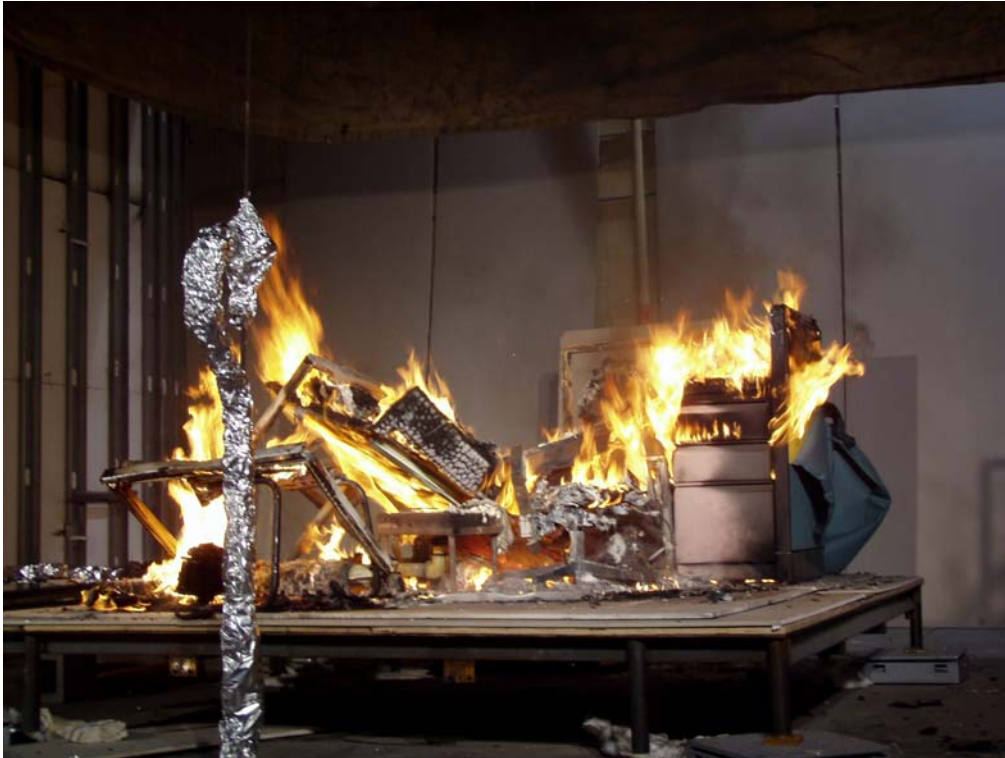
Figure 70. Single workstation at 930 s after ignition
