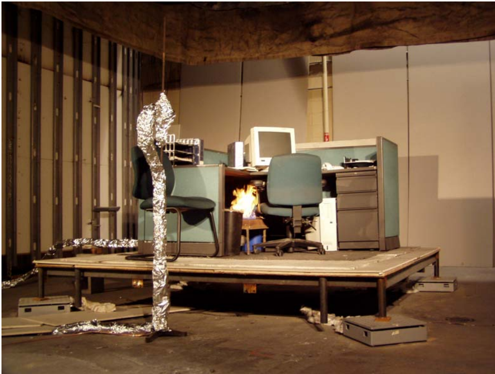
Figure 67. Single workstation a few seconds after the ignition of the gas burner
