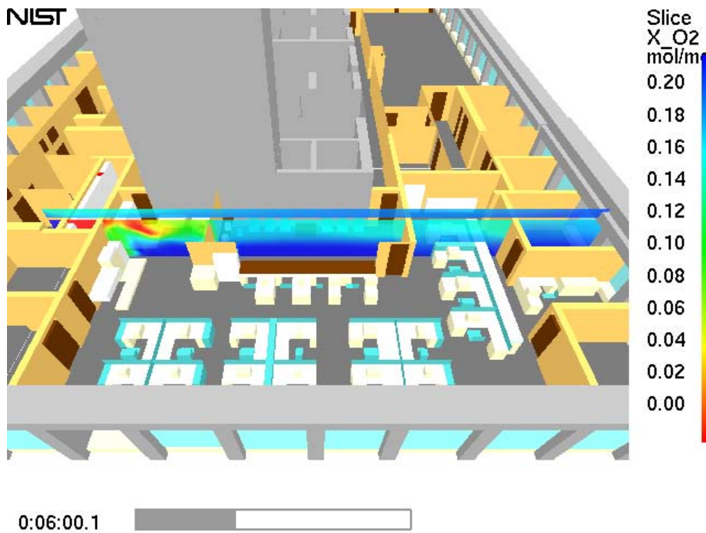
Figure 116. Oxygen concentration, 360 s (6 min)
