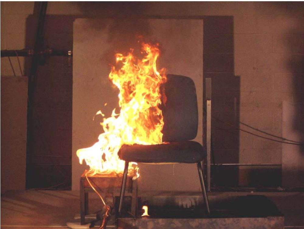
Figure 47. Sled base chair, approximately 90 s after ignition
