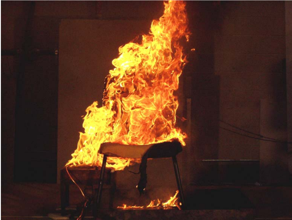
Figure 48. Sled base chair, approximately 150 s after ignition
