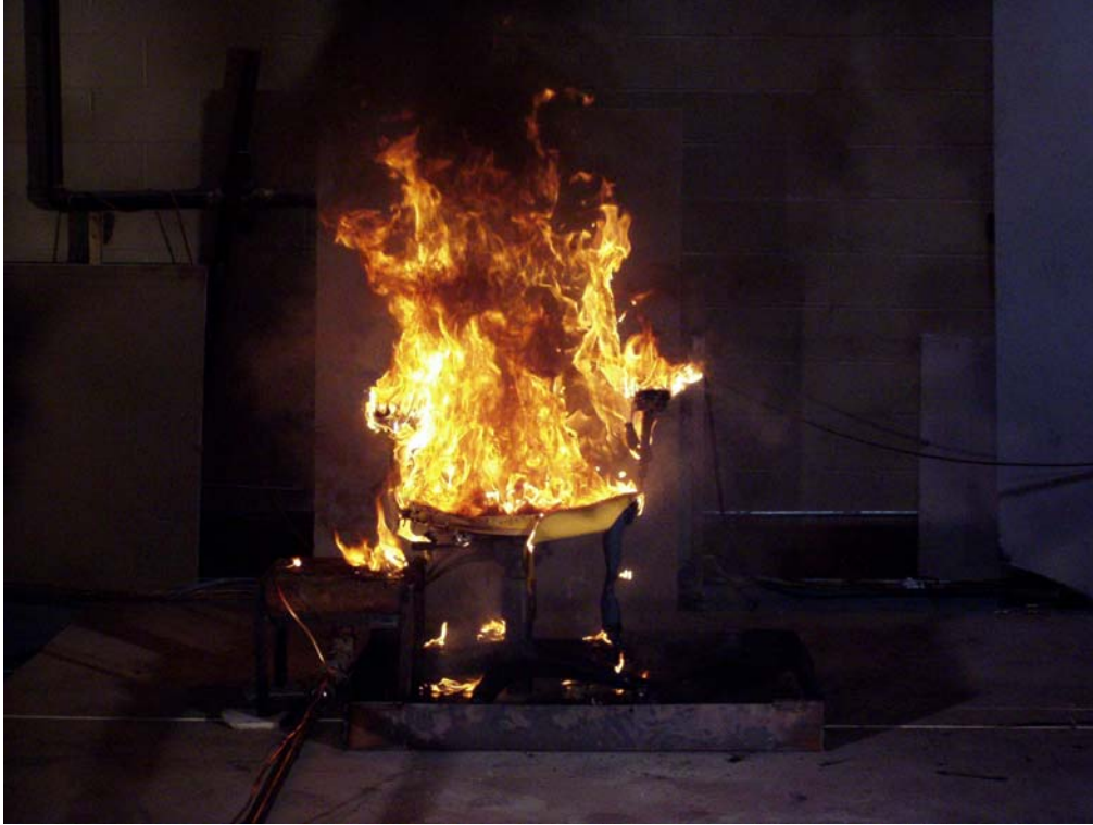
Figure 56. Office chair, approximately 210 s after ignition, near first peak HRR
