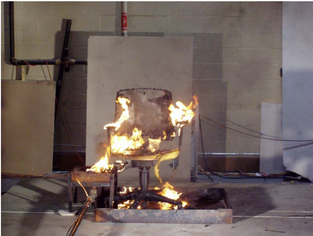
Figure 57. Office chair, approximately 380 s after ignition
