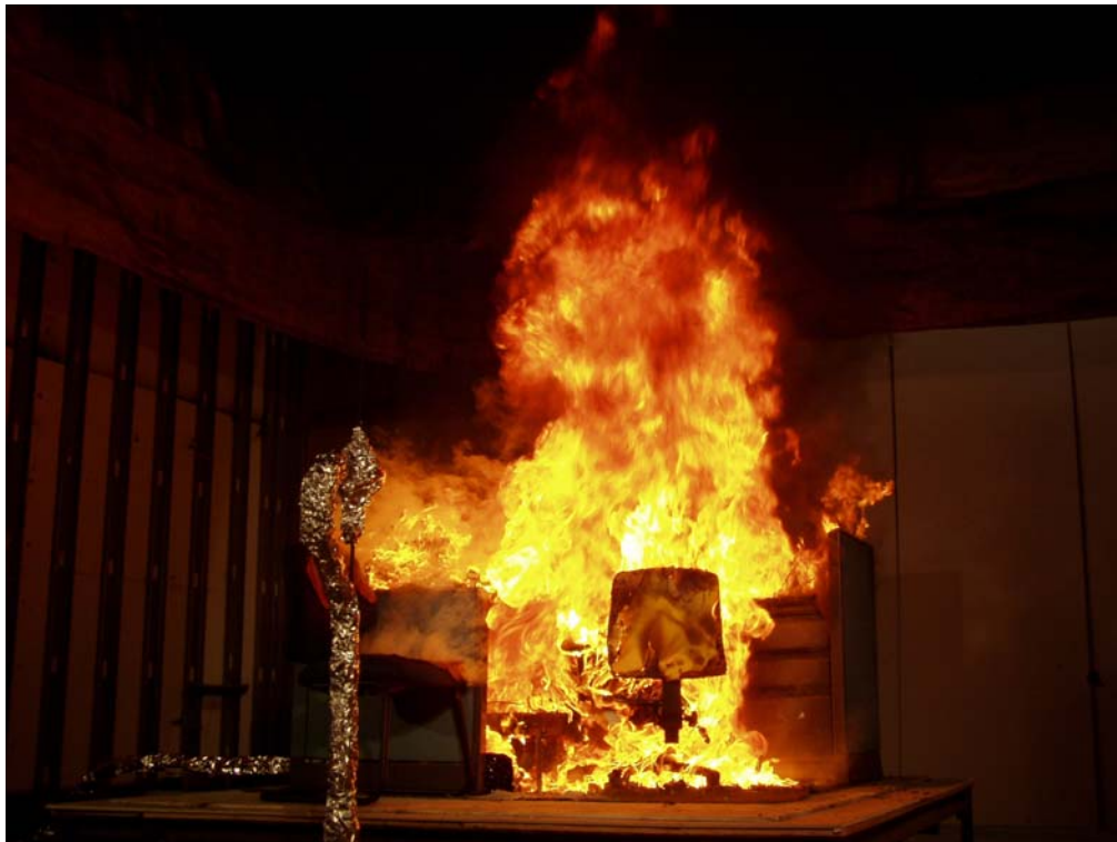
Figure 69. Single workstation, 360 s after ignition, near peak HRR of 3.3 MW
