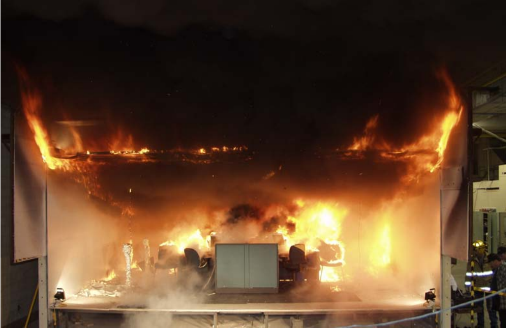
Figure 83. View of the enclosure, approximately 300 s after ignition
