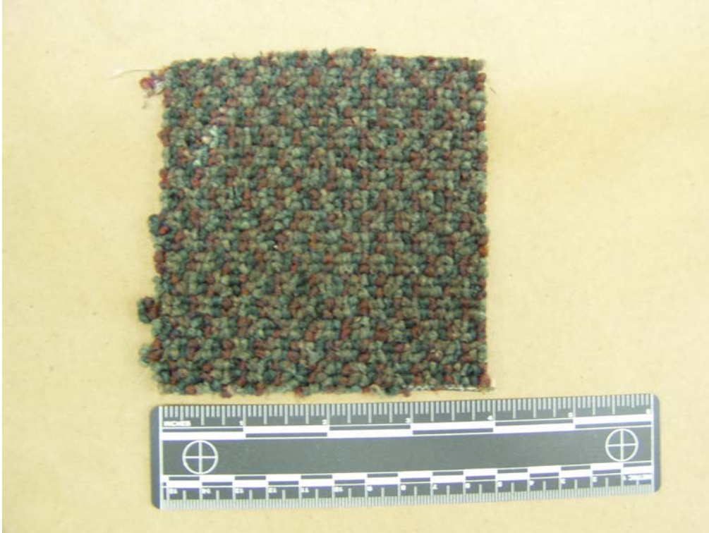
Figure 29. Photograph of carpet sample cut for testing in the cone calorimeter
