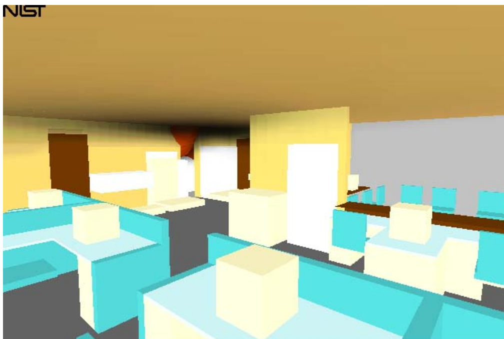
Figure 131. Smoke at 120 s (2 min)
