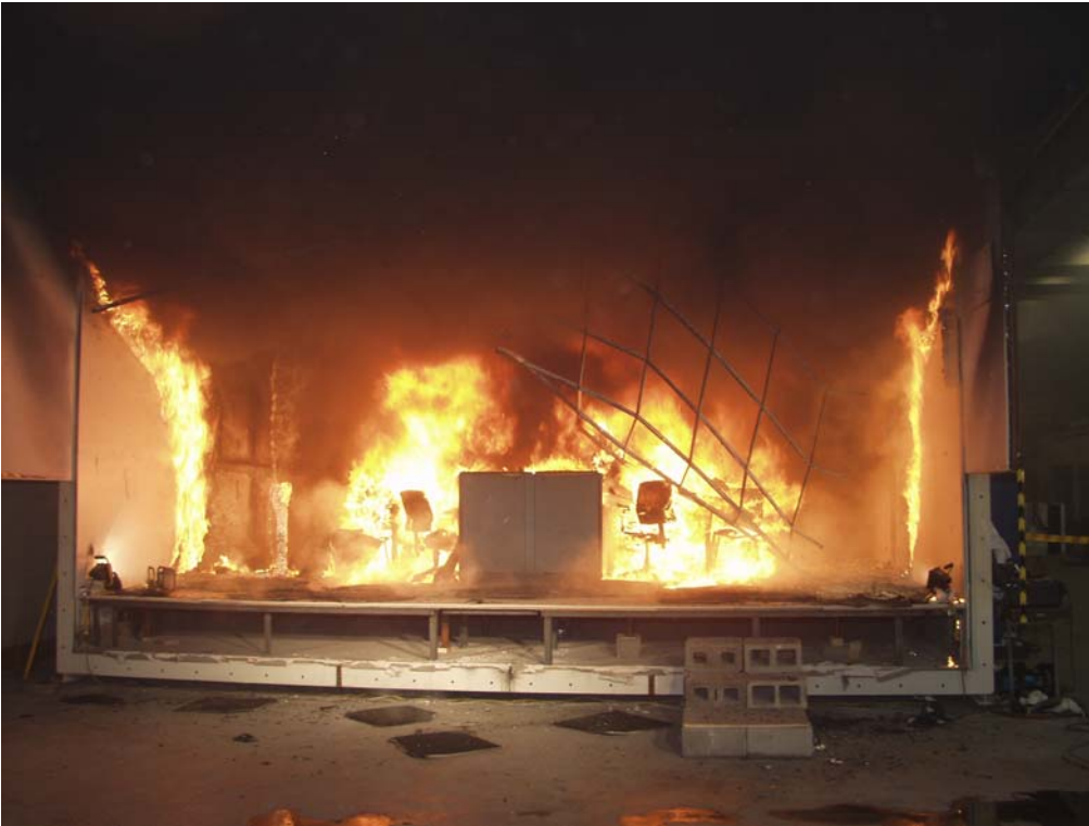
Figure 84. View of the enclosure, approximately 430 s after ignition
