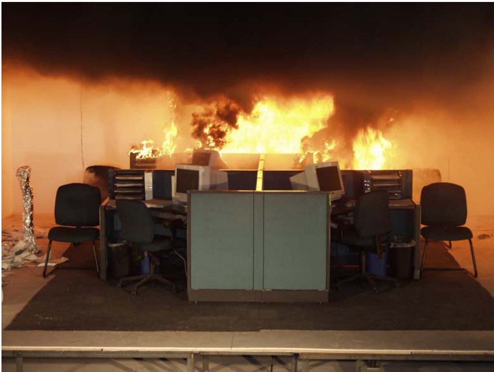
Figure 82. View of the enclosure, approximately 180 s after ignition
