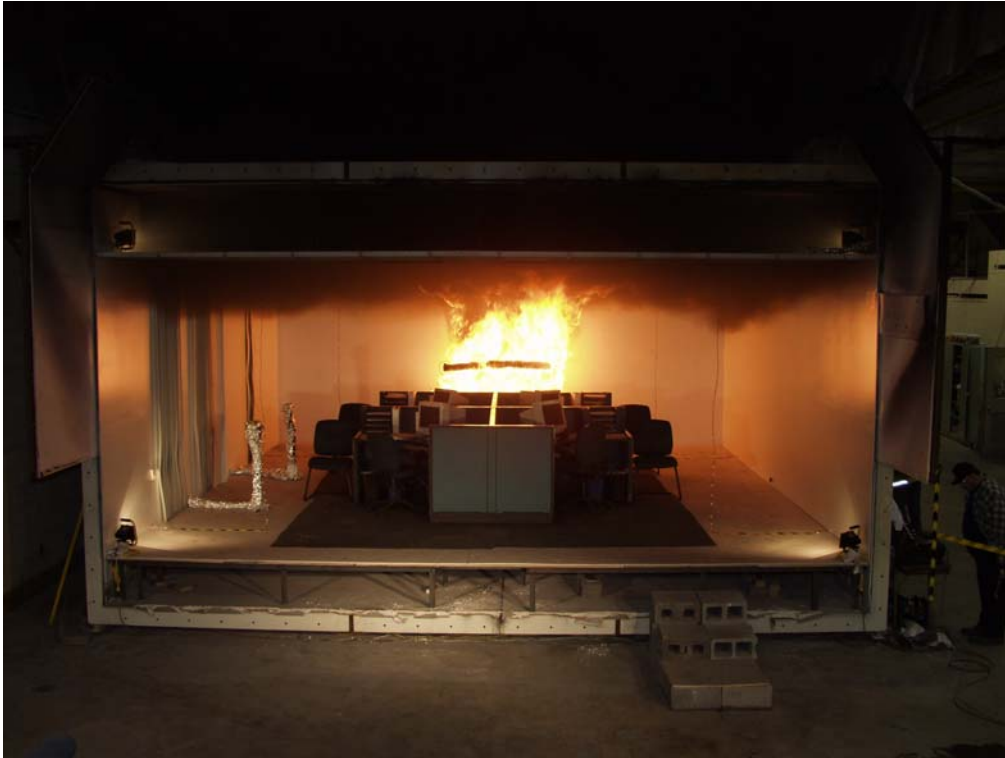
Figure 81. View of the enclosure 20 s after ignition of the burners
