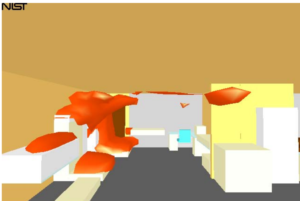
Figure 113. Flame iso-surface at 242 s (4 min 2 s), inside view
