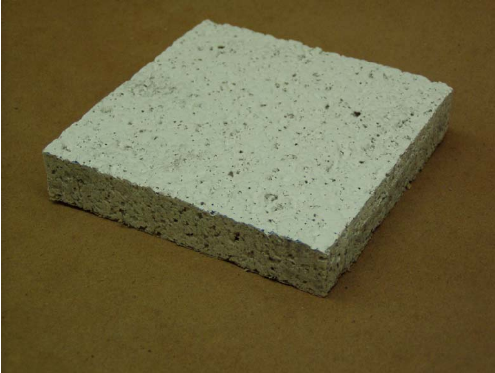
Figure 30. Photograph of a piece of ceiling tile, shown with finished surface facing up
