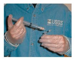
Figure 2. Hexavalent chromium field separation.
