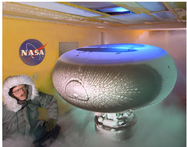
A full-size aircraft component, such as this helicopter radar housing, is being tested in the Icing Research Tunnel.
