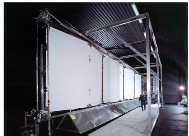
Radiator testing in Space Power Facility
