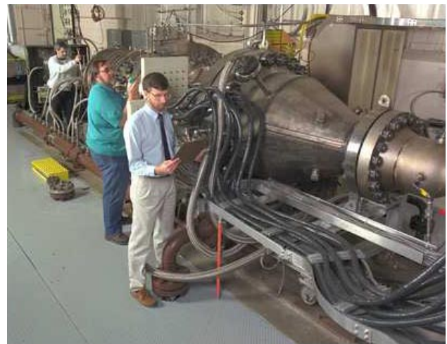
The Advanced Subsonic Combustion Rig is a state-of-the-art facility for analyzing and fine-tuning the performance of aircraft engine combustors.
