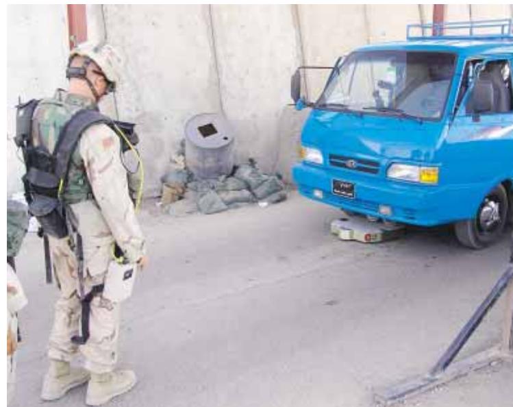
▲ A Soldier in Iraq uses a thin, lightweight robot known as an ODIS to conduct an under-vehicle inspection.
