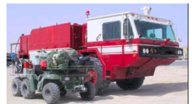
Aircraft Crash and Rescue Fire Fighting (ARFF) vehicle [right] and First Response Expeditionary (FRE) vehicle [left].
