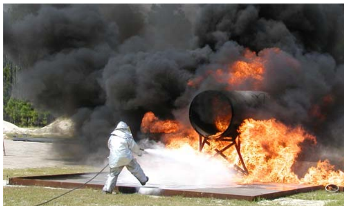
Evaluating the High Pressure Fire Extinguishment in 3-D F 100 engine nacelle fire simulation at Tyndall AFB
