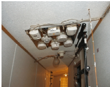
Residential detector sample test board used in study.
