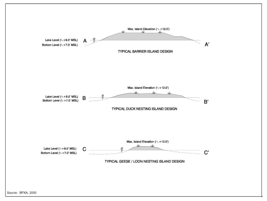
Figure II.C-9 Duck Island Mine Site - Proposed Restoration - Typical Cross-Sections
