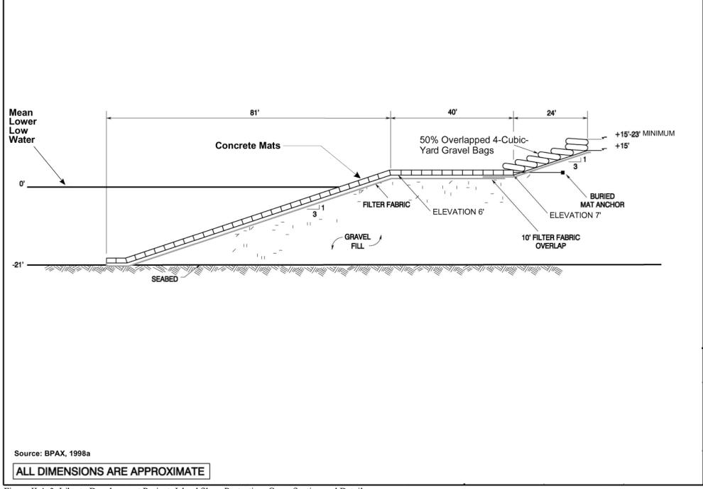
Figure II.A-3 Liberty Development Project: Island Slope Protection, Cross-Section and Details
