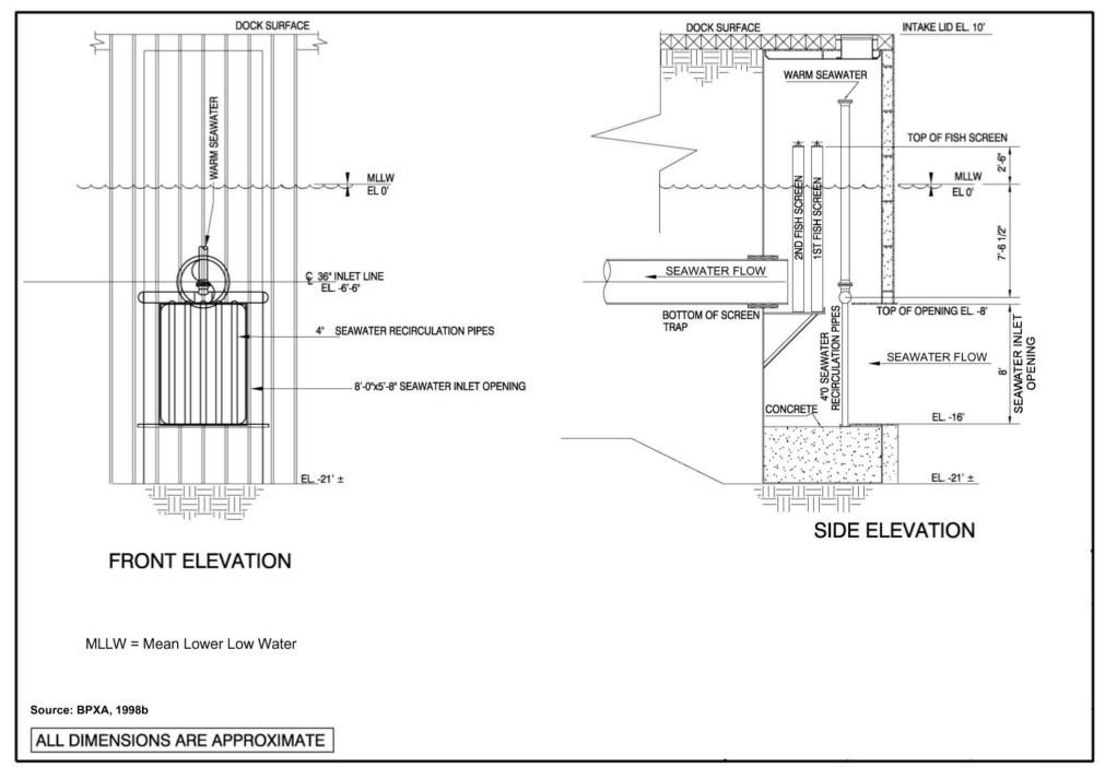
Figure III.D-1 Liberty Development Project: Seawater Intake Detail
