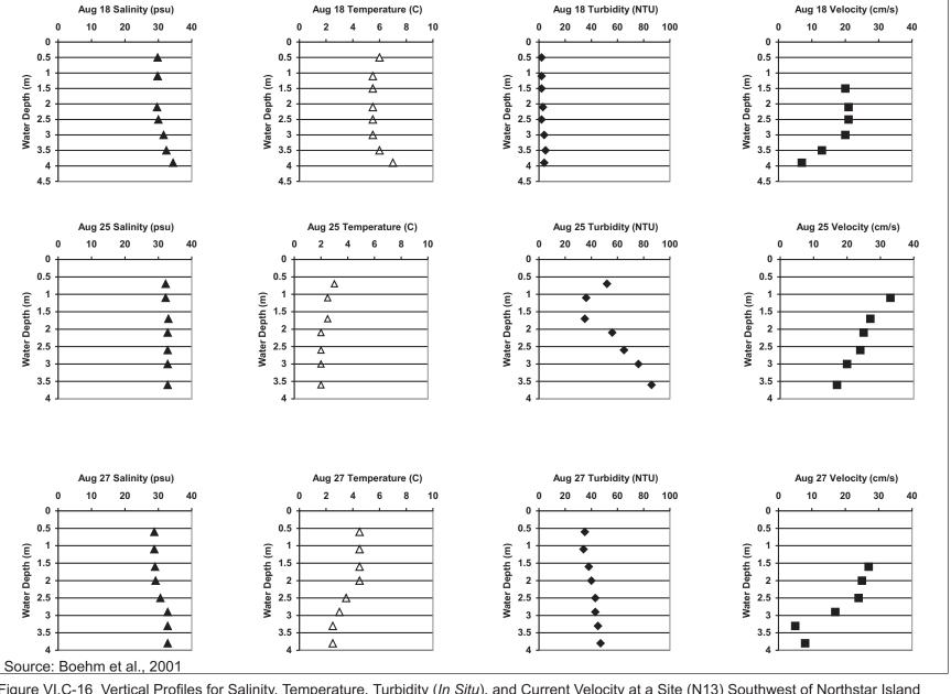
Figure VI.C-16 Vertical Profiles for Salinity, Temperature, Turbidity (*In Situ*), and Current Velocity at a Site (N13) Southwest of Northstar Island during 1999 before and after Storm Conditions
