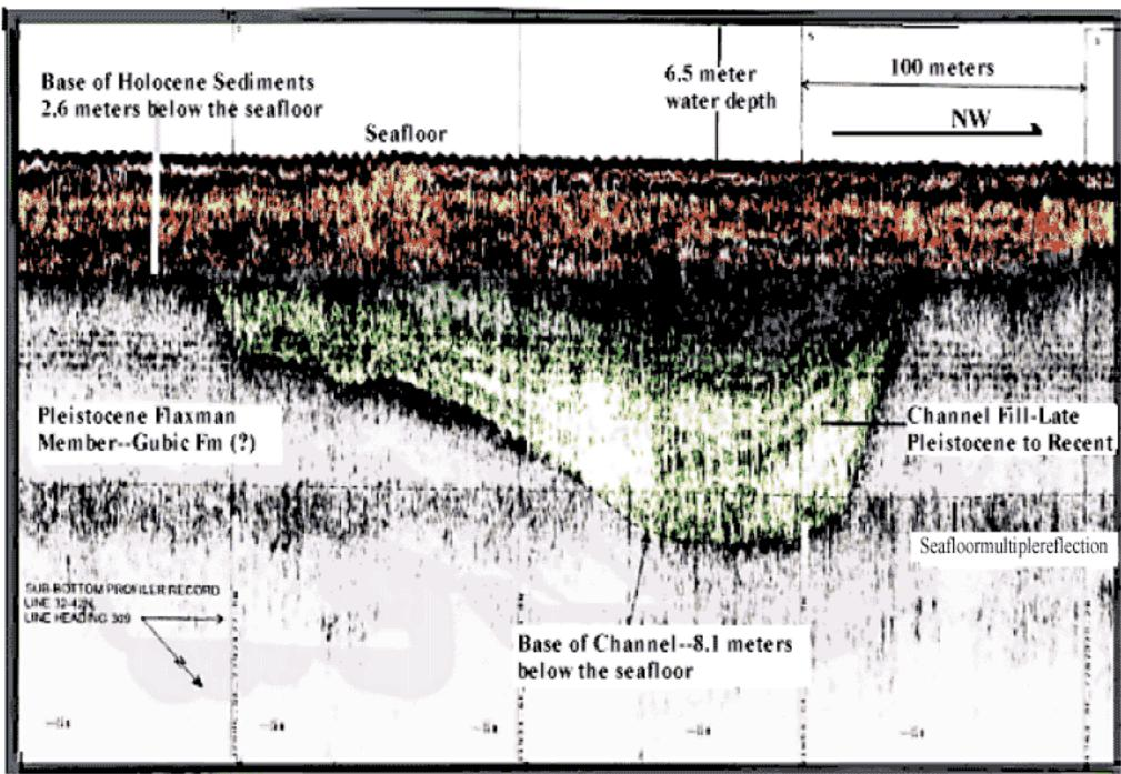
Figure VI.C-10 "Chirp" high-resolution seismic profile records showing a submerged buried Pleistocene or Holocene channel. At a lower sea level, the channel cut into Pleistocene sedients approximately 5.5 meters. After sea level rose, it was drowned and subsequently covered by 2.6 meters of Holocene marine sediments. Record from Watson Company Liberty Site survey.
