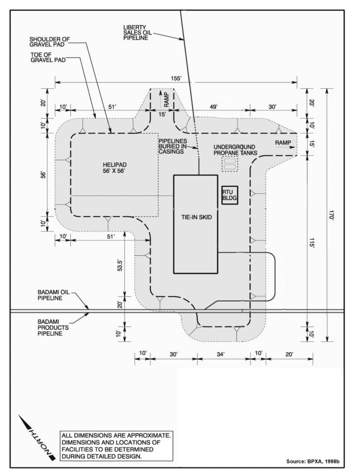
Figure II.A-16 Liberty Devolopment Project: Pad at Badami Pipeline Tie-In, Plan View
