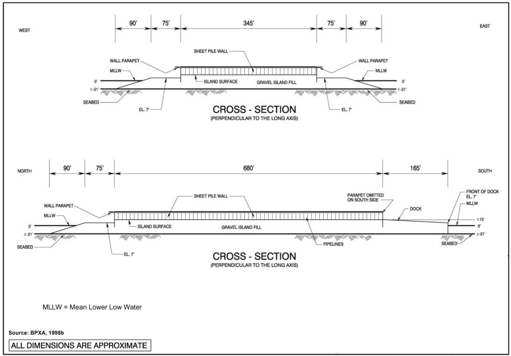
Figure II.C-4 Liberty Development Project: Sheet Pile Island (Alternative IV), Cross Sections
