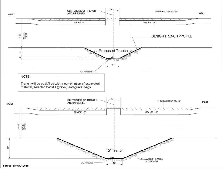
Figure II.C-10 Liberty Development Project: Comparison of Proposed Trench (Alternative I) and 15-Foot Deep Trench (Alternative VII)
