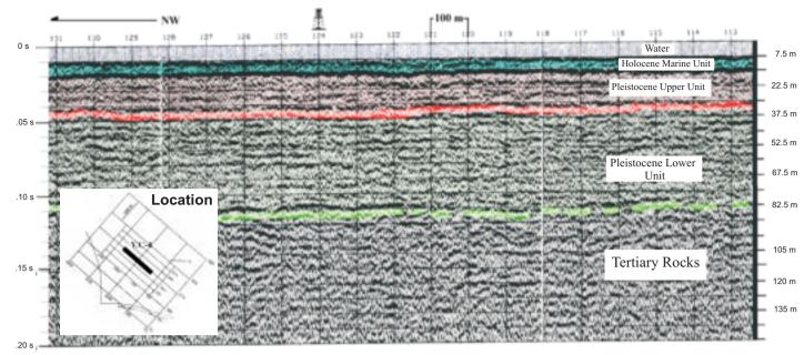
Figure VI.C-4 Minisparker profile record passing through the island site, showing Pleistocene and Holocene stratigraphic units overlying strata of Tertiary age. The uppermost unit, interpreted as Holocene marine sediments, is mapped on a regional scale in Figure VI.C-2. The seismic stratigraphic horizon between the Pleistocene upper and lower units is correlative to "Seismic Horizon 3" of Dinter et. al (1990) shown in Figure V.C-5. Minisparker record from Watson Company Liberty Site Survey.
