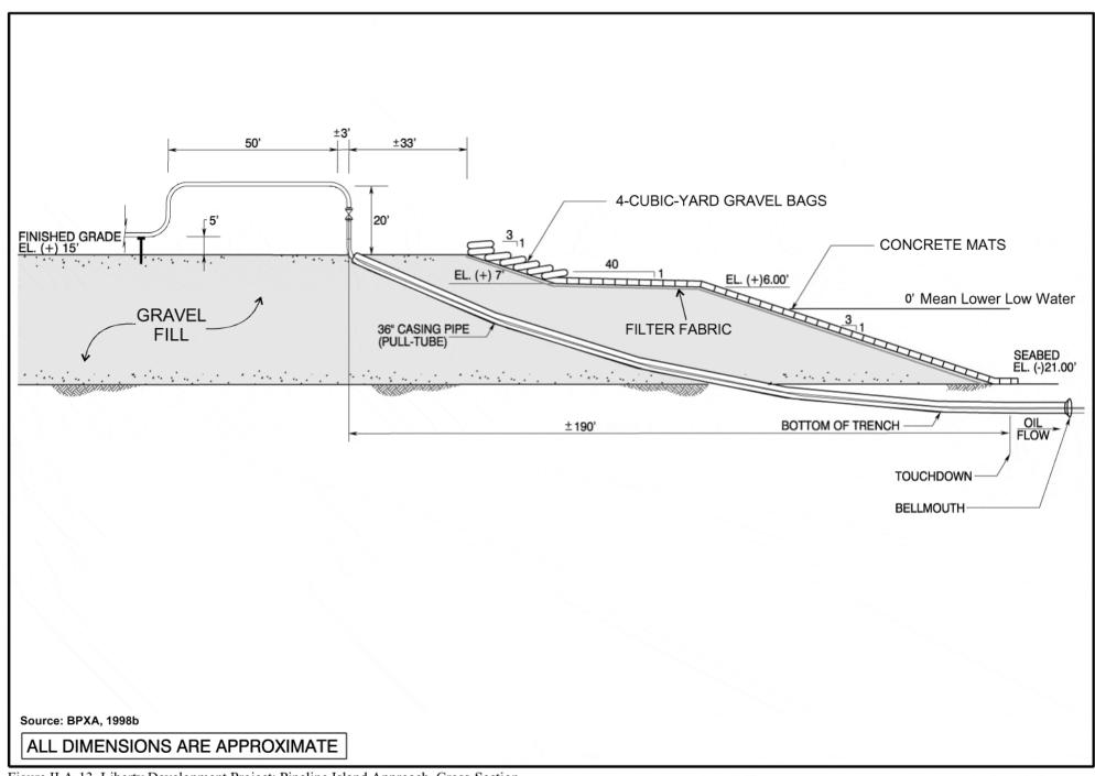
Figure II.A-13 Liberty Development Project: Pipeline Island Approach, Cross-Section
