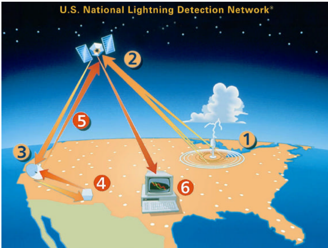
How the NLDN works: 1) Sensors transmit data to satellite; 2) Satellite relays information to earth station; 3) Data is transmitted to NCC via landlines; 4) NCC processes data; 5) Processed data is relayed back to satellite; 6) Lightning data is displayed within seconds of occurrence.
