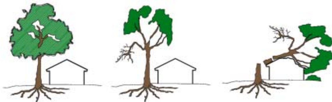
Fig. 16: Trees planted too close to the home can be a source of structural damage. Root systems might crack foundation walls, creating a path for water infiltration.
