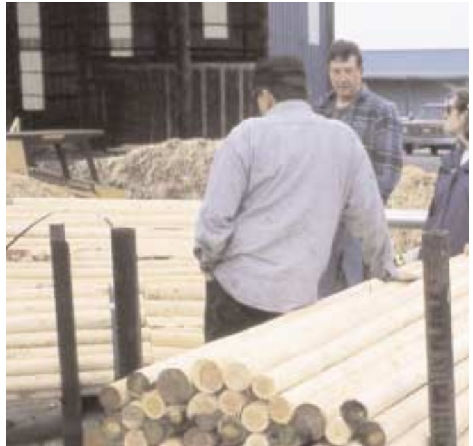
Manufacturing small logs into posts and rails for fencing at the Jefferson State forest products mill in Hayfork, California.
