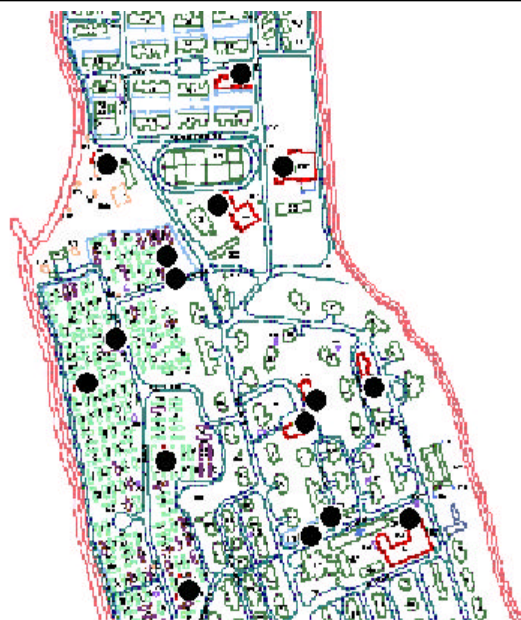
Figure of the XYZ Water System Showing the Spatial Location of Consumer Complaints. The darkened circle indicates the location of one consumer complaint that has been filed in the last 24 hours.
