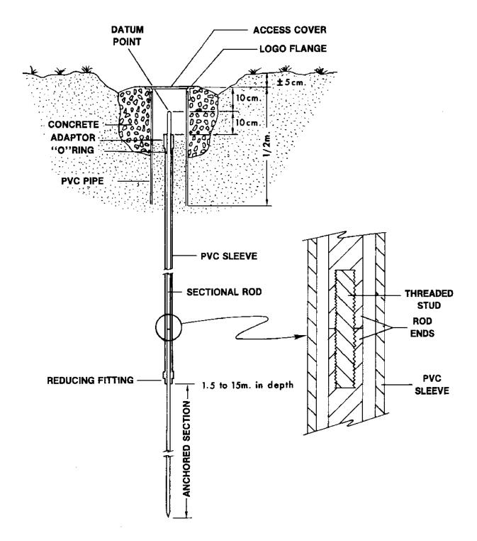
Figure 4.-Sleeved class A rod mark.
