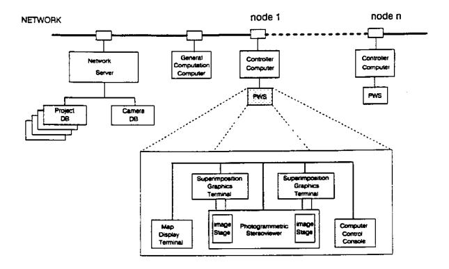
Figure 3.--IDPF system architecture.
