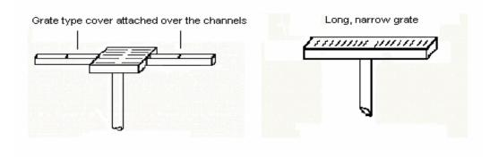
Figure 2. Alternate Drain Configurations
