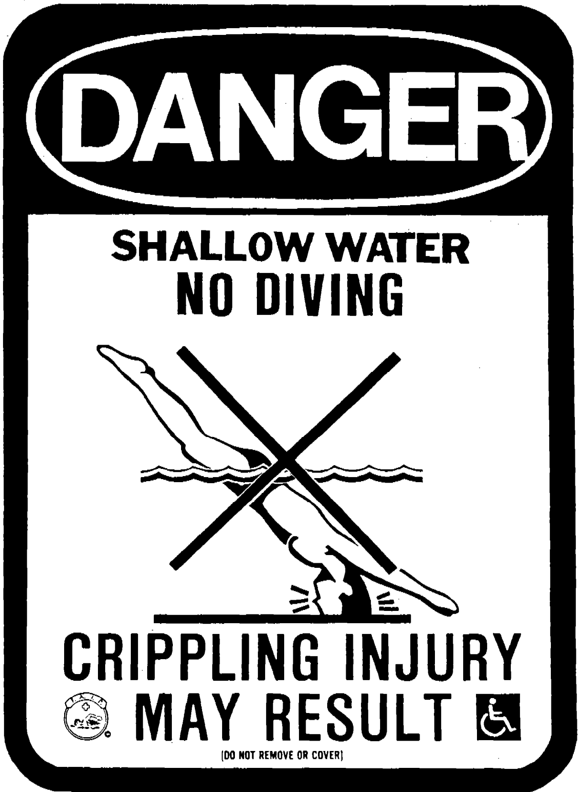
Figure 6-2. A typical sign which should be posted in areas having a water depth less than 5 ft (1.5 m). The word DANGER should have a bright red contrasting background. This sign may be reduced to a 4 in. by 6 in. sign and mounted on the coping of the swimming pool.
