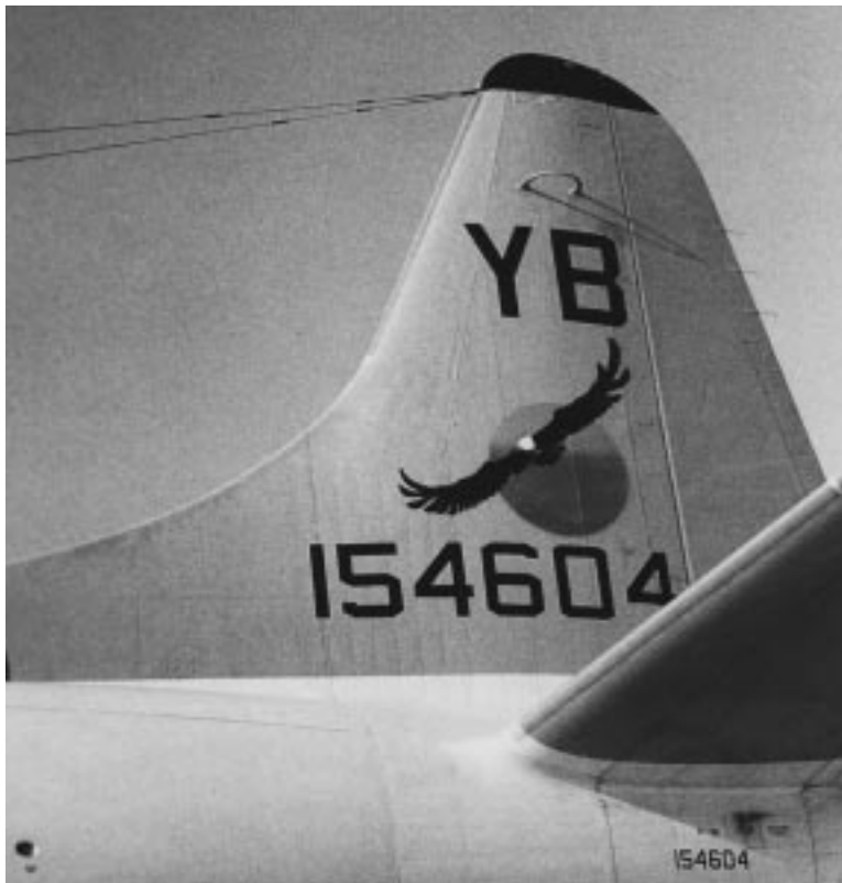
The Bureau Number for this P-3 Orion is in big numbers, 154604, on the tail and small numbers on the rear of the fuselage. The photo also shows the squadron's insignia and its tail code, YB.
